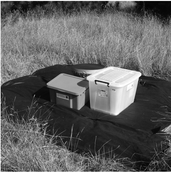
Fig. 1. A bioacoustic unit situated in rank grass. The 2 containers in the foreground house the laptop (left) and the ceramic pot placed behind.
