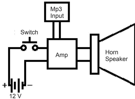
Fig. 1. Wiring diagram of the broadcast system components.
